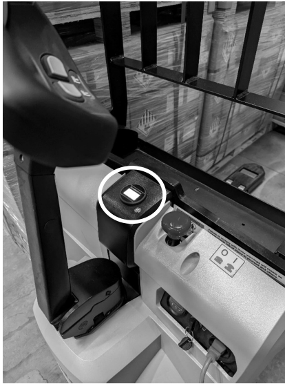
Figure 7. BDI Display installed on a Walkie Pallet Jack
