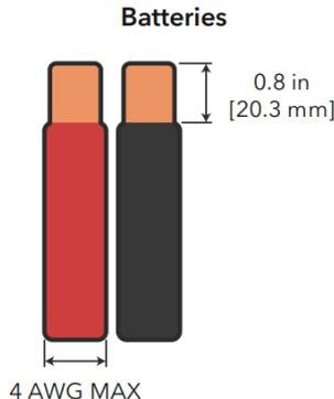
Figure 29. Battery Cables
