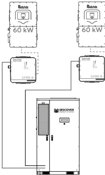
Figure 12. Inverter - LYNK II - Cabinet Communication
