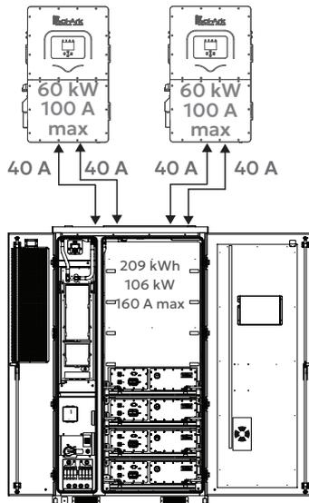
Figure 9. Two Inverters, One Cabinet Connection
