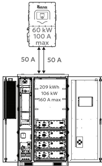
Figure 14. One Inverter, One Battery Connection
