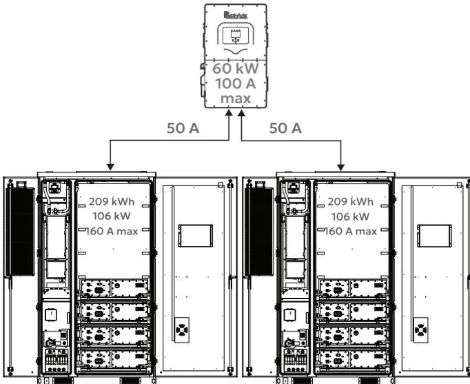
Figure 19. Inverter - Cabinet Connection
