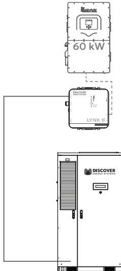
Figure 17. Inverter - LYNK II - Battery Communication
