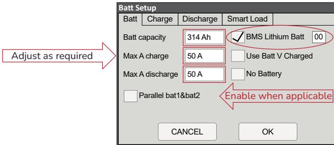
Figure 34. Batt Setup - Batt Tab
