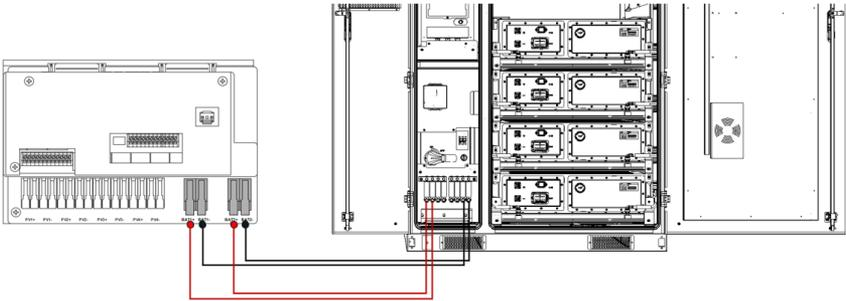
Figure 16. Inverter to Cabinet DC Wiring
