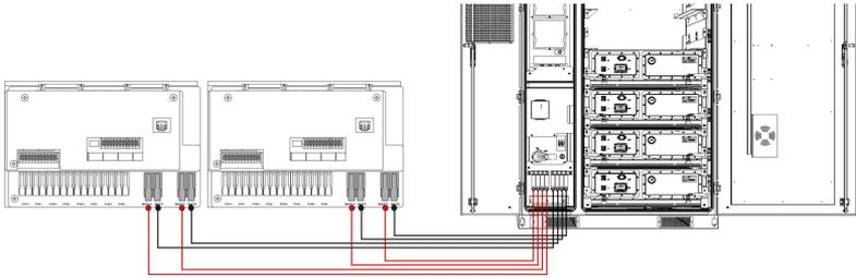
Figure 11. Inverter to Cabinet DC Wiring
