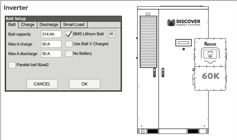
Figure 36. 60 kW/209 kWh - One 60K-3P Inverter, One AES 210HV Battery Cabinet
