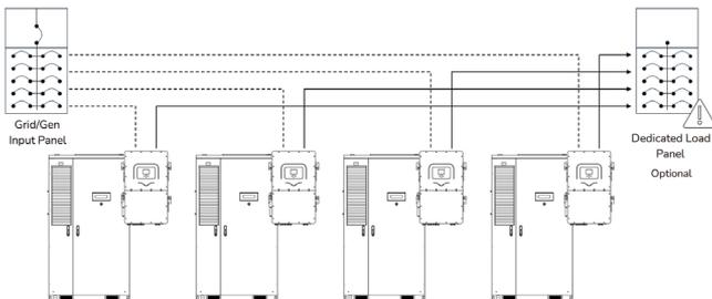
Figure 7. Parallel Multiple Sol-Ark 60K-3P on the AC Bus (up to 10 inverters)
