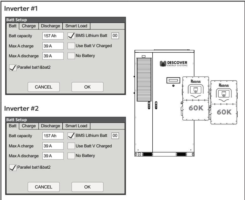
Figure 35. 120 kW/209 kWh - Two 60K-3P Inverters, One AES 210HV Battery Cabinet
