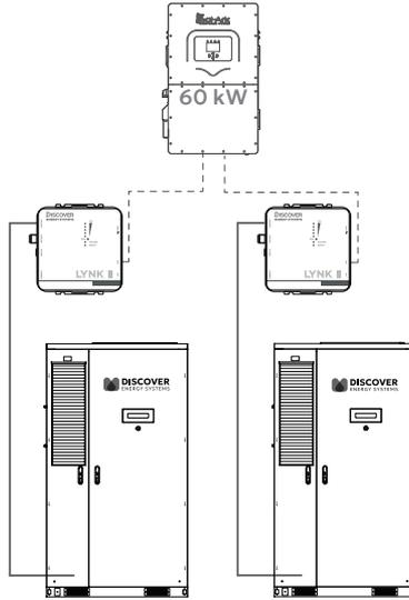
Figure 22. Inverter - LYNK II - Cabinet Communication
