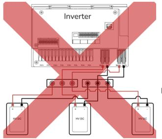
Figure 6. Do Not Parallel Battery Cabinets on the DC Bus
