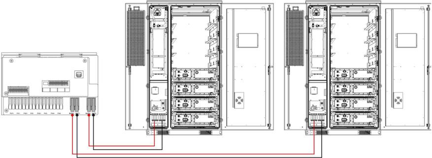
Figure 21. Inverter to Cabinet DC Wiring
