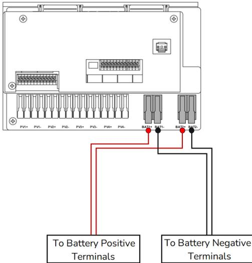
Figure 23. Multi-Terminal Installation
