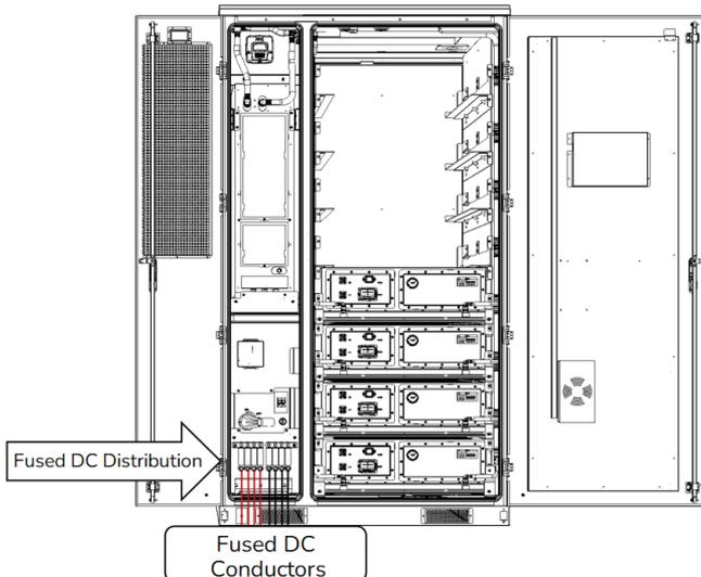
Figure 2. DC Distribution Box Wiring
