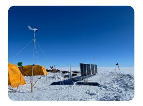
Power from the system runs a multitude of sensors and electrical measurement equipment, including the Automatic Surface Flux Station (ASFS), Ground Penetrating Radar (GPR), Micro Rain Radar (MRR), Microwave Radiometer (MWR), Ice Mass Balance (IMB), Open GNSS Research Equipment (OGRE), Portable Optical Particle Spectrometer (POPS), as well as other electronics.
