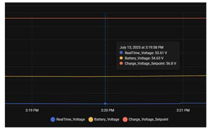
RealTime\_Voltage = BMS Closed Loop Voltage (and measured DC Bus Voltage)
